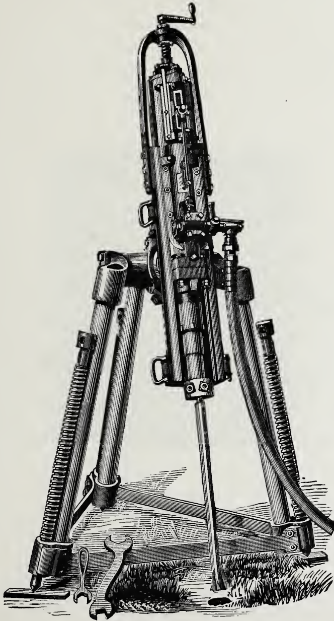
Fig. 1.—Drill Mounted on Iron Tripod for Rock-Cutting.
